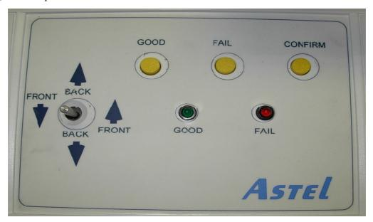
The GOOD and FAIL keys are enabled with a double LED flash when one of the keys is pressed, the LED under the button is activated to ask the operator to confirm the choice by pressing the CONFIRM key on the console panel.
