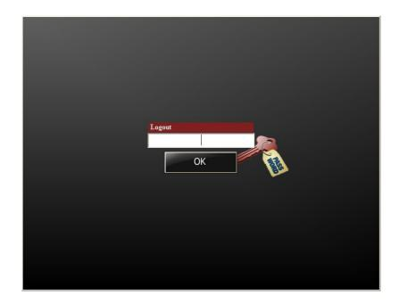
If password is not correct, the system will not be allowed to restart under Windows. If password is correct, system will reboot under Windows. A special procedure have to be followed shutting down Windows to restore machine at the next restart.
