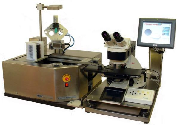
System is computer controlled, and its use and programming is really easy and user friendly. It is possible, if needed, to edit and recall recipes, and each recipe includes inspection strategies (all wafers, fixed wafers and random access for statistical inspection) and handling parameters. Proteus Macro Inspection is mounted on a vibration free granite base, and can be supplied also with different kinds of inspection lamps for any different need.
