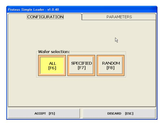
If the SELECTION mode is selected, only specified wafers will be inspected, and these wafers must be selected in a further screen as follows, by selecting it with up/down arrows and by pressing, the ENABLE or DISABLE key (only clicking).
