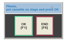
Cassette mapping will then be started to identify wafers into cassette. When mapping is finished, machine will wait for the microscope stage in exchange position. The screen displayed at this time will include the graphics indication of wafer found in cassette. Type of inspection active will be the same given int the recipe. It is possible to modify this selection before starting the cycle.
