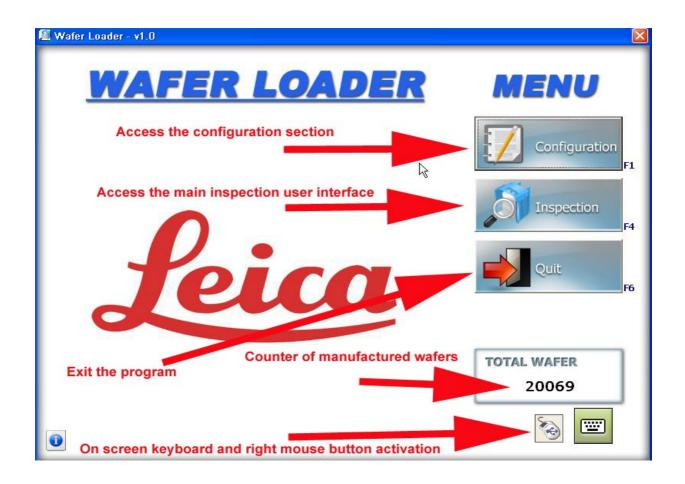
To run the inspection, press the INSPECTION button, will then run the next interface, which is the proper user interface.
